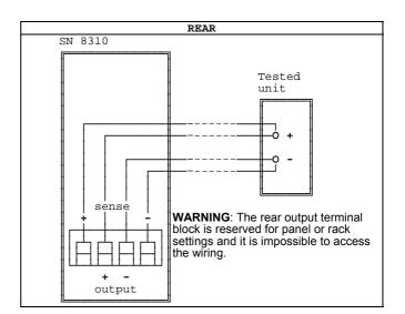
Avoid any stray e.m.f and minimize the resistance of the connection wires to the sense terminals.
