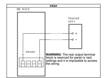
With the 2-wire configuration, voltage present on SENSE terminals of the SN 8310 is that programmed. Select the connection wires according to the specifications of the tested unit.
